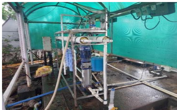
RO System Covered by Polycarbonate Housing
